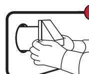
From the outside, slide pipe through the hole opening until the vent is flush against outside wall surface.
