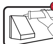
Secure to outside wall using 4 screws (Not Included). Caulk around vent and outside wall if necessary.
